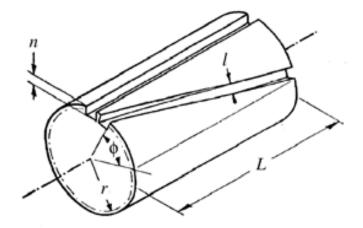
If the speed is  $v = \omega L/\phi$  then the molecule gets through the slot.
