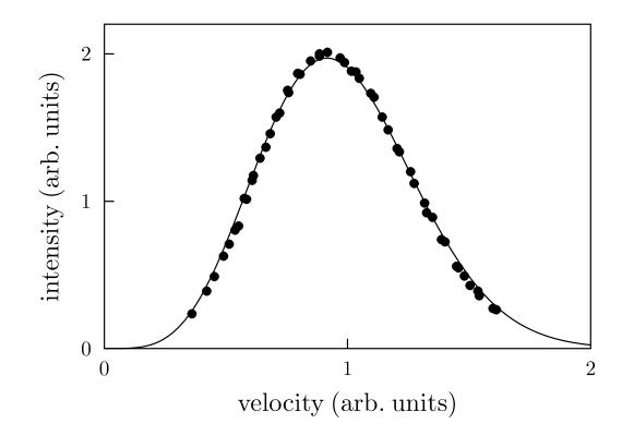
Fig. 5.7 Intensity data measured for potassium atoms using the velocity selector shown in Fig. 5.6 (from R. C. Miller and P. Kusch, Phys. Rev. 99, 1314 (1955), Copyright (1955) by the American Physical Society). The line
